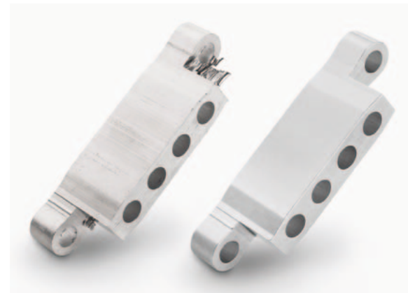
Work piece before and after deburring
