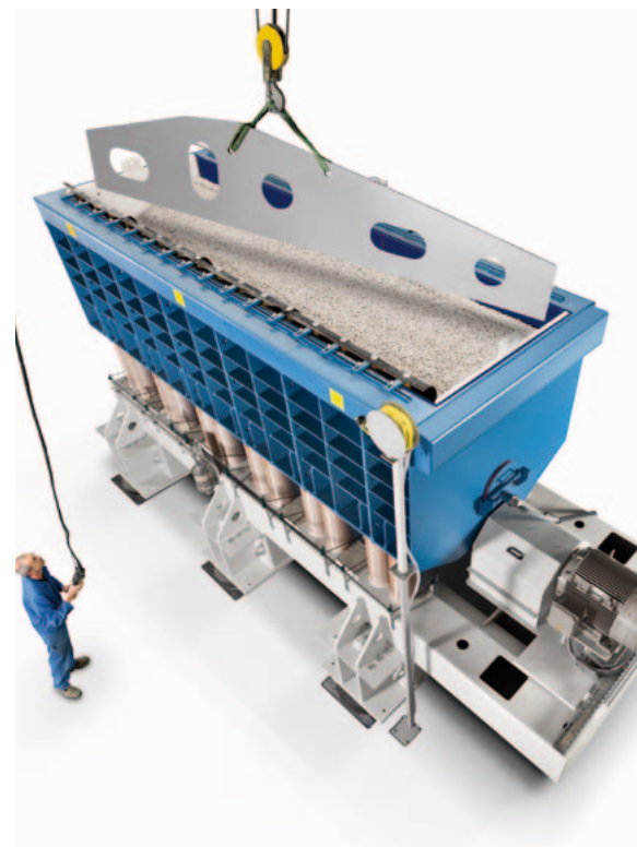
Tub vibrator, model range TMV, for up to 5,000 mm long work pieces
