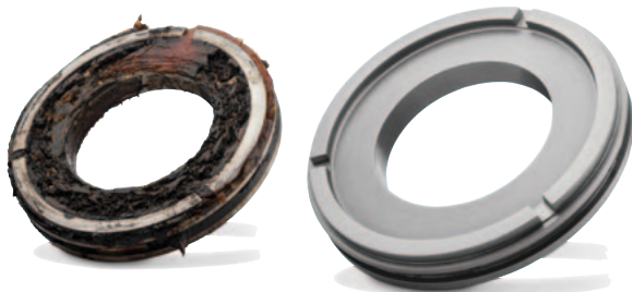
Work piece before and after de-oiling/degreasing
