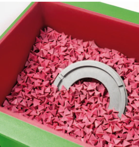
Processing of spacer disks in a tub vibrator
