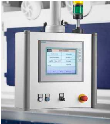
Operator panel of a THM shot blast machine with touch screen
