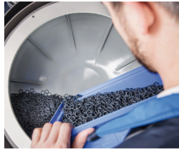
The Rotamat systems can be used for coating of mass produced small parts, for example, made from elastomers (photo) or metal.
